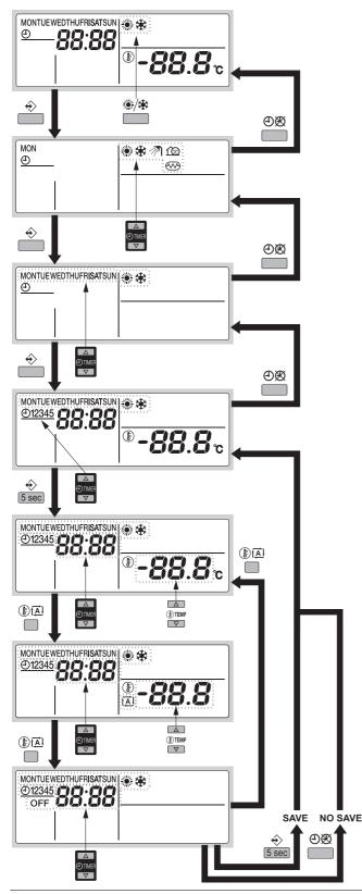
NOTE Programming space cooling or space heating are both done in the same way. At the start of the programming procedure space cooling or space heating is selected. After that, you have to return to the start of the programming procedure to program the other operation mode.
