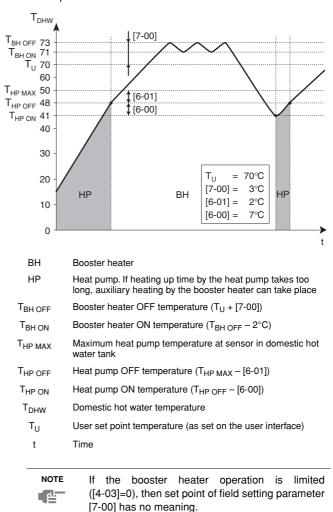
■ [7-00] Domestic hot water step length: temperature difference above the domestic hot water set point temperature before the booster heater is turned off.
